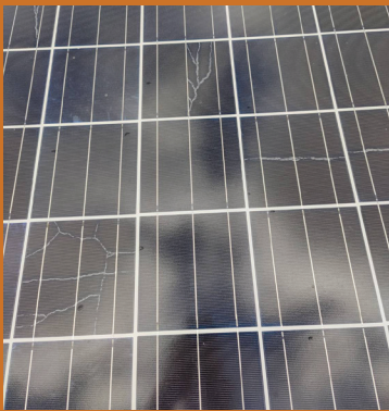
Micro Cracks on a Solar Panel
